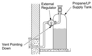
Figure 39 - External Regulator with Vent Pointing Down (Propane/LP Only)
